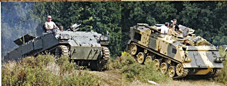
Above right: the Abbot self-propelled gun (left) is based on the running gear of the FV432 APC seen here on the right of the photo.
